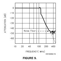
*Figure 9* shows the large signal sine wave frequency response of the LM2403. The frequency response rolls off very rapidly above the bandwidth limit of the amplifier. There are two reasons for this fast response roll-off:
