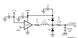
FIGURE 10. One Channel of the LM2403 with the Recommended Arc Protection Circuit
